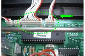
Remove the Control wire or located as indicated in this picture.
