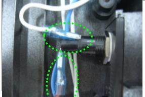
With hold the body of Fuse holder, Remove the as indicated in this picture.
